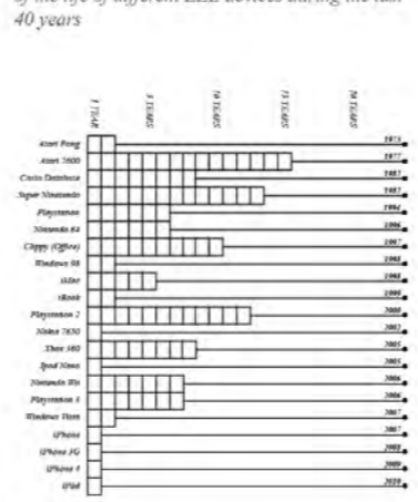
Fig.85. Planned obsolescence diagram: evolution of the life of different EEE devices during the last 40 years
