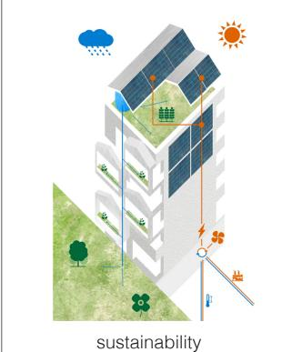
It generates its own energy with air, geothermal heat pumps and pv panels, and reuses rain for plants rather than directly draining it.
